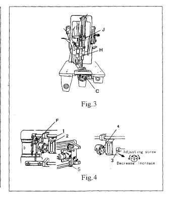
Lubrication of rotating hook (Fig. 4)
