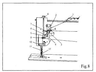
into the fork 5, in the thread controller. Guide upward through the point of controller discs 6, and thread guide 7, and from right to left through the eye in take-up lever 8, down through thread guide 7, again and then through 9, 10, 11 and from left to right through the eye of the needle 12.
