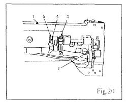
foot must be adjusted. To adjust this, lower the presser bar lifter, holding the vibrating presser foot B (Fig.6) and loosen the hexagon screw 3 and move the presser foot up or down as may be required. After setting the position, tighten the screw.
